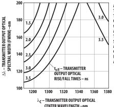
AFBR-5803 FDDI TRANSMITTER TEST RESULTS OF  $\lambda_{C}$ ,  $\Delta\lambda$  AND type Correlated and comply with the allowed spectral width as a function of center wavelength for various rise and fall times.
