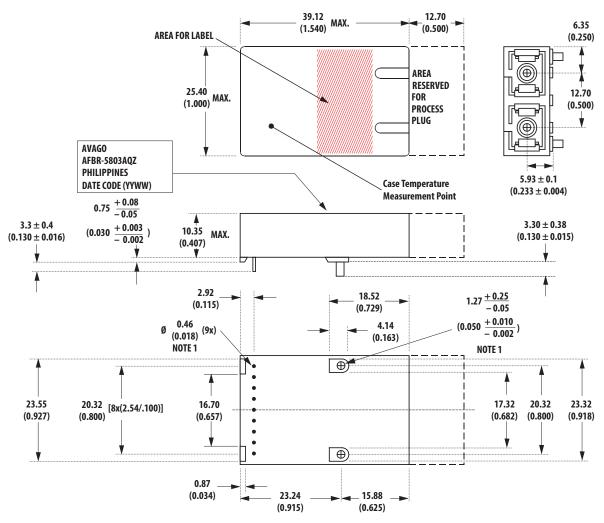
Note 1: Phosphor bronze is the base material for the posts & pins. For lead-free soldering, the solder posts have Tin Copper over Nickel plating, and the electrical pins have pure Tin over Nickel plating.
