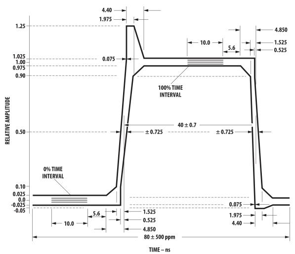
THE AFBR-5803 OUTPUT OPTICAL PULSE SHAPE SHALL FIT WITHIN THE BOUNDARIES OF THE PULSE ENVELOPE FOR RISE AND FALL TIME MEASUREMENTS.
