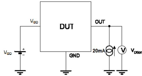
Note 1 - The output saturation voltage  $V_{DSon}$  is measured at  $V_{DD}=3.8V$  and  $V_{DD}=24V$
