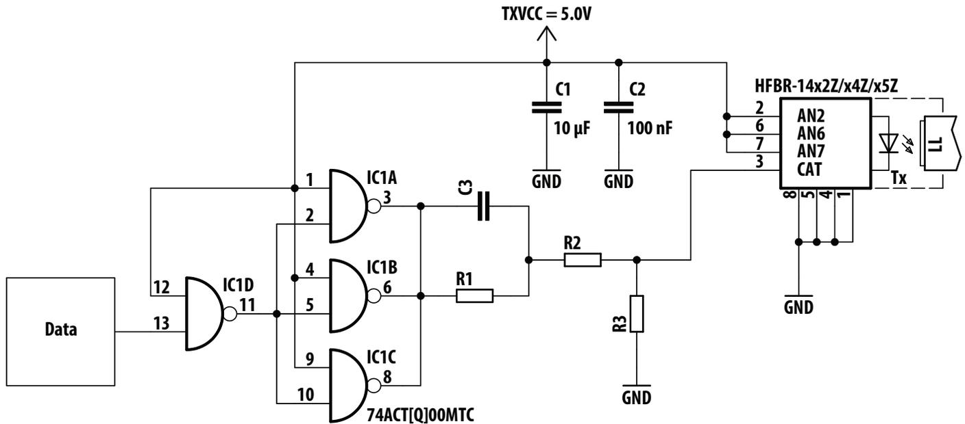
**NOTE:** The component values shown in the table create a typical driver current of 60 mA (peak). An individual check of the optical output signal quality of the used optic transmitter is recommended during the circuit design.
