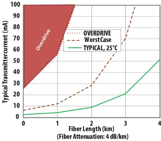
Figure 4: Typical HFBR-14x4xZ/HFBR-24x2xZ Link with 62.5/125 μm Fiber
