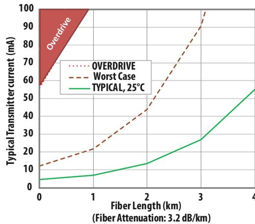
Figure 5: Typical HFBR-14x4xZ/HFBR-24x2xZ Link with 50/125 μm Fiber
