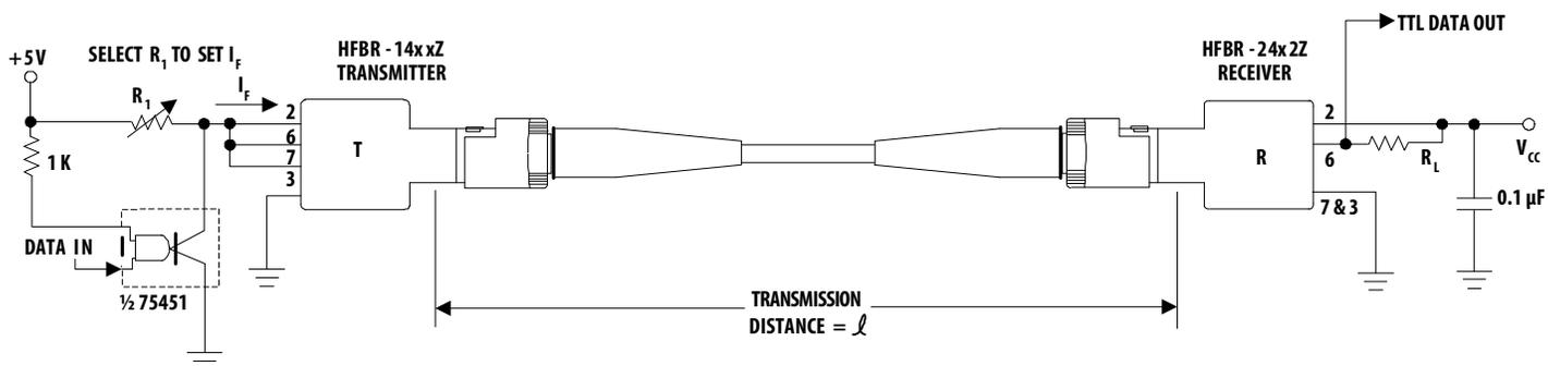
**NOTE:** A bypass capacitor (0.01  $\mu\text{F}$  to 0.1  $\mu\text{F}$  ceramic) must be connected from pin 2 to pin 7 of the receiver. Total lead length between both ends of the capacitor and the pins should not exceed 20 mm.
