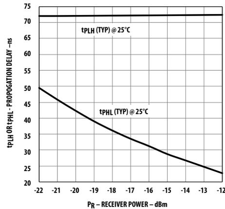
Figure 7: Typical Pulse Width Distortion of Link (HFBR-14x4Z/ HFBR-24x2Z) measured at T<sub>A</sub> = 25°C, 5 MBaud, and with 1m of Cable
