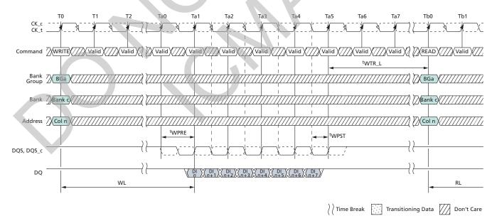
Notes: 1. <sup>t</sup>WTR\_L: delay from start of internal write transaction to internal READ command to the same bank group.
