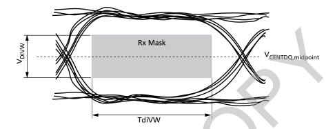
$V_{CENTDQ,midpoint}$  is defined as the midpoint between the largest  $V_{REFDQ}$  voltage level and the smallest  $V_{REFDQ}$  voltage level across all DQ pins for a given DRAM. Each DQ pin's  $V_{REFDQ}$  is defined by the center (widest opening) of the cumulative data input eye as depicted in the following figure. This means a DRAM's level variation is accounted for within the DRAM Rx mask. The DRAM  $V_{REFDQ}$  level will be set by the system to account for  $R_{ON}$  and ODT settings.
