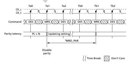
Notes: 1. <sup>t</sup>MRD\_PAR = <sup>t</sup>MOD + N; where N is the programmed parity latency.
