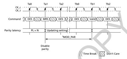
Notes: 1. <sup>t</sup>MOD\_PAR = <sup>t</sup>MOD + N; where N is the programmed parity latency.
