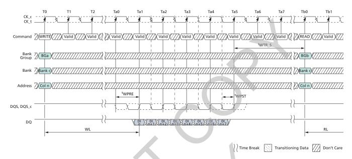
Notes: 1. <sup>t</sup>WTR\_S: delay from start of internal write transaction to internal READ command to a different bank group.
