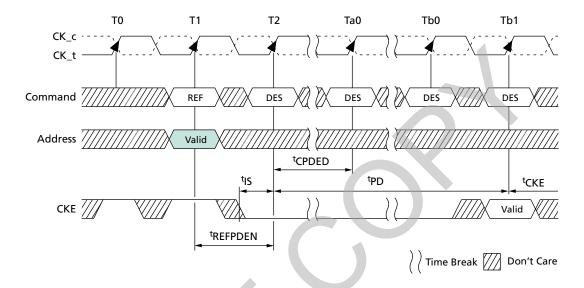
Figure 95: Active Command to Power-Down Entry
