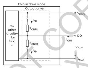
The output driver impedance,  $R_{ON}$ , is determined by the value of the external reference resistor  $R_{ZQ}$  as follows:  $R_{ON(34)} = R_{ZQ}/7$ , or  $R_{ON(48)} = R_{ZQ}/5$ . This provides either a nominal  $34.3\Omega \pm 10\%$  or  $48\Omega \pm 10\%$  with nominal  $R_{ZQ} = 240\Omega$ .
