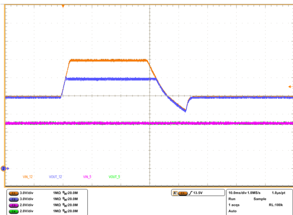
Figure 33. Voltage clamp during operation (12 V eFuse)
