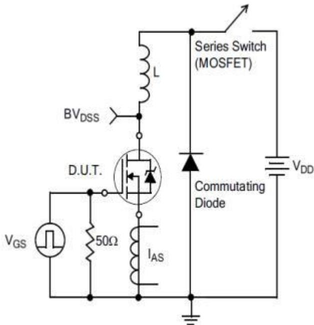
Figure G. Unclamped Inductive Switching Test Circuit
