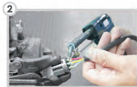
使用夾具將接頭夾持住，線材裸線與上固定體的接觸體缺口進行焊線加工 Using the clamp to fix the connector, doing soldering assembly between the bar wire and upper body.
