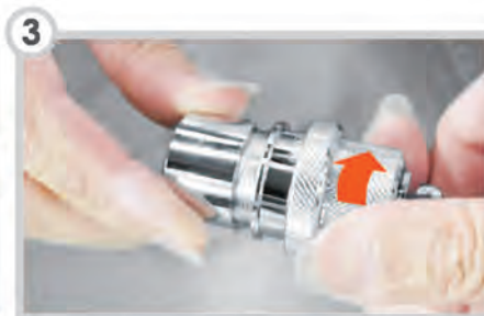
本體與上固定體對鎖，將螺紋順時針方向鎖緊(需轉動本體鎖入，非轉動接頭) The body and upper one are locked together. Screw clockwise and be sure to only rotate the body itself instead of the whole connector.
