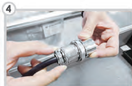
半月邊壓入(與線材不能留有間隙) Crescent-shaped clamp mounted ( The gap couldn't be allowed with the cable connected )
